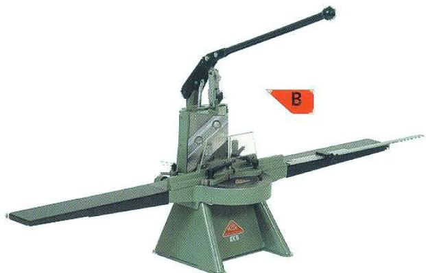
Bench Model ideal for glazing beads etc. to be cut in one cut. The machine is operated by a hand lever which is very easy to push down due to the carefully prepared construction. Morsø-B is supplied with table extensions to both sides and knives.
