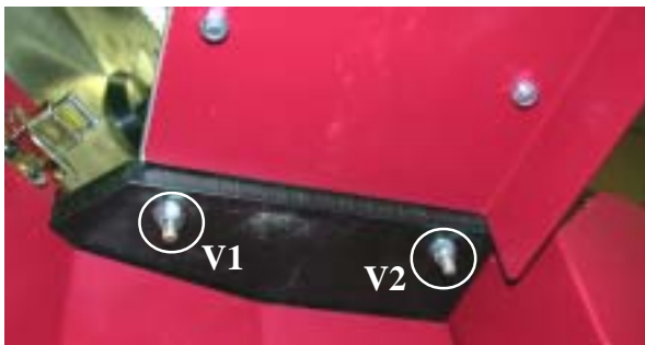
Retighten screws V1 and V2 below the table.
